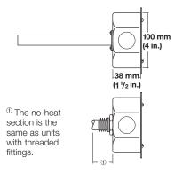
NEMA 1, NEMA 4 (moisture-proof) and NEMA 7 (explosion-proof) octagonal terminal boxes can be mounted to a flange or threaded fitting on the 12.5, 16 and 20 mm diameter units. These 100 mm (4 in.) terminal boxes have conduit knockouts to protect electrical connections.
