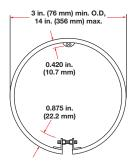
Two fiberglass-insulated lead wires rated to 840°F (450°C) exit a metal braid 180° opposite from gap, Type B outside diameter designed and constructed to mate with inside diameter of cylinders. Maximum width for outside diameter heaters is 6 in. (152 mm). To order, specify **outside diameter and width** of heater.
