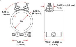
Post terminals provide optimum connections. Screw thread is 10-24. To order, specify **post terminals** (metric threads available).
