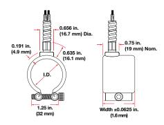
Type H: A flexible steel hose encloses the leads for maximum abrasion protection. Leads are 2 in. (51 mm) longer than hose. Shipped with 12 in. (305 mm) leads, unless longer length is specified. To order, specify **Type H** and **length.**
