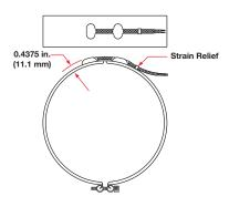
Two fiberglass lead wires exit a single, tightly woven metal braid at a right angle on the expandable construction vs. two sets of leads. The minimum diameter capability is 4 in. (102 mm). Minimum width capability is  $1^{1/2}$  in. (38 mm). To order, specify **Type SLE** and **length.**
