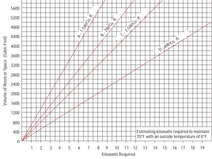
Curve A — Rooms with little or no outside exposure. No roof or floor with outside exposure; only 1 wall exposed with not over 15% door and window area.
