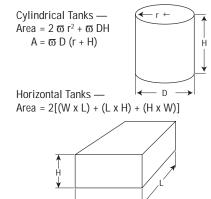
Tank Tracing Example — Maintain a metal tank with 2 inch thick Fiberglas® insulation at 50°F. The tank is located outdoors, is 4 feet in diameter, 12 feet long and is exposed at both ends. The minimum ambient temperature is 0°F and the maximum expected wind speed is 15 mph.
