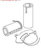
To increase heating efficiency of your application, silicone rubber heaters can be thermally insulated with silicone sponge rubber bonded to one side in the following thicknesses: 1/16, 1/8, 1/4, 3/8 or 1/2 in. (1.6, 3.2, 6, 9.5 or 13 mm).
