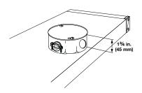
To protect electrical connections, a standard NEMA octagon terminal box is available. The standard size is  $3^9/16 \times 3^9/16 \times 1^1/2$  in. (90.5 x 90.5 x 38 mm) with knockouts for  $^1/2$  in. (13 mm) conduit. Other NEMA sizes are available as an extended capability.
