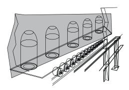
Watt densities can be varied across the entire width of RAYMAX heaters. If desired, each zone can have an individually controlled power supply.
