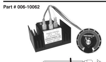
The Power Control Module offers infinitely variable phase control when used with resistive loads up to 25 amps. The solid state circuitry provides modified transient suppression, exceptional stability and life. An external potentiometer/switch (dial plate and knob included) is used to control output voltage. A trimming potentiometer is mounted on top of the module to adjust turn on voltage level. This device should be installed in a circuit fused at 120% rated load or 30 amps maximum.
